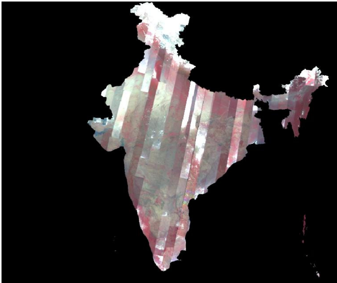
Figure 1. HYSI Radiance Image Mosaic of Indian subcontinent (FCC combination: Band 40 - Red, Band 30 - Green, Band 20 - Blue)
